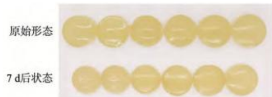
图 10 储存 7 d 形态对比 Fig.10 Comparison of morphology after 7 days of storage
